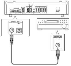
AV amplifier or receiver with built-in Dolby Digital, DTS, or MPEG decoder
